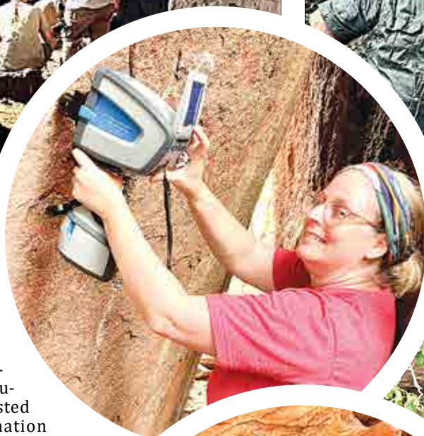
The archeologists carried out analyses to uncover the materials behind the ancient paint. Using a portable X-ray device and handheld Raman machines that beam lasers, they examined the Bushman paintings up close.
